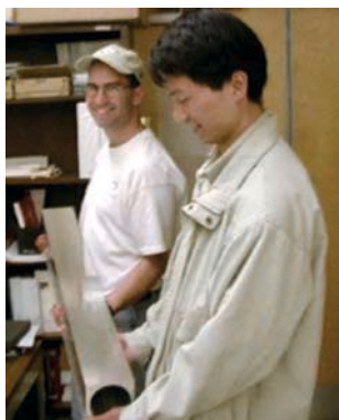
The EXES echelon grating was diamond-machined by Hyperfine, Inc. from a single piece of 6061 Aluminum. It measures 4" x 40" and weighs 25 lb.
