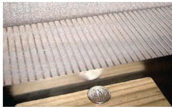
A closeup of the EXES echelon grating. The groove spacing is 7.6 mm and the angle of incidence is 84.3 degrees. The design of EXES is based upon our successful TEXES spectrograph (see http://arXiv.org/abs/astro-ph/0110521 ).
