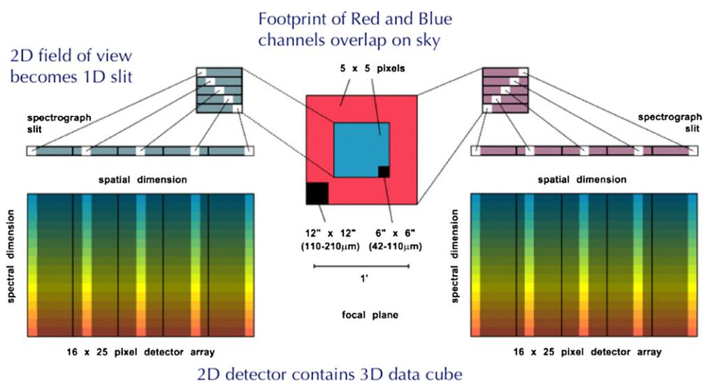
**Figure 6.** Imaging spectroscopy of FIFI-LS. The  $5 \times 5$  spatial pixels in both the red and the blue channel are each optically rearranged to form a long slit before entering the red and blue grating spectrometer. The correct arrangement of the pixels will be reestablished during data reduction to form a data cube. (FIFI-LS Team<sup>©</sup>).
