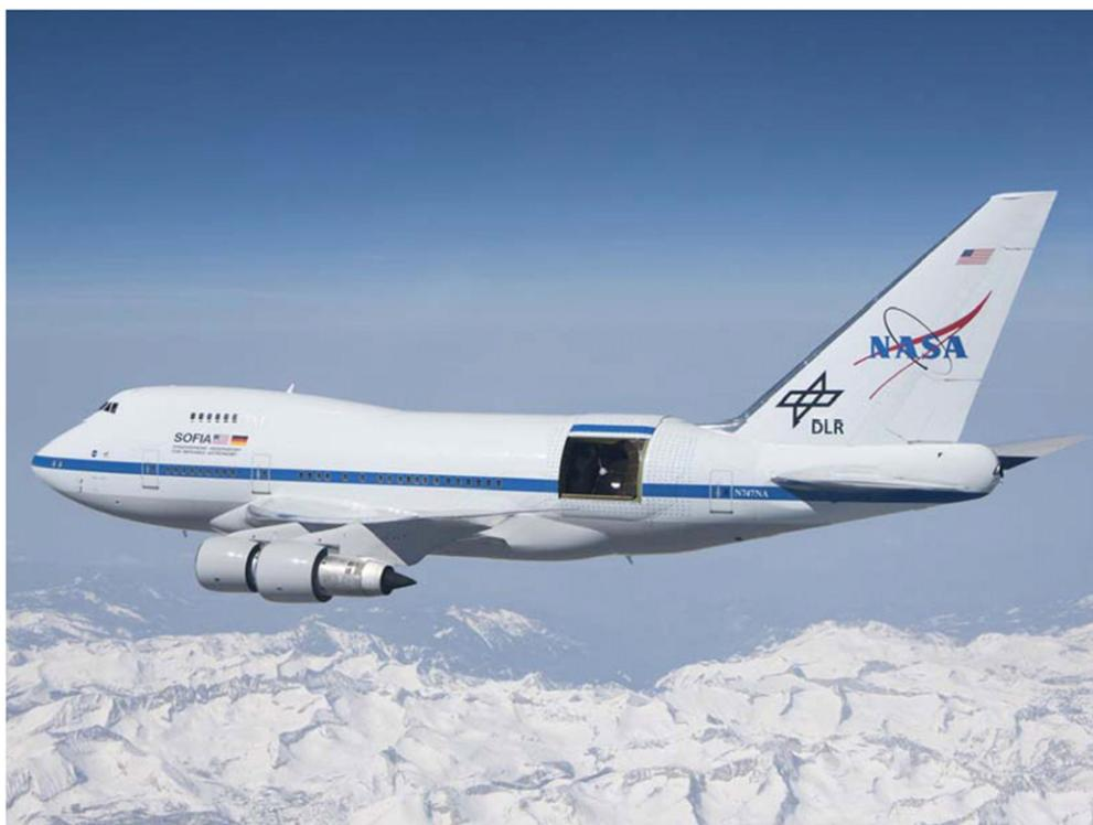
**Figure 2.** With the sliding door open showing its 17-ton infrared telescope, SOFIA soars over California's snow-covered Southern Sierras on a test flight on 14 April 2010 (NASA<sup>©</sup>).
