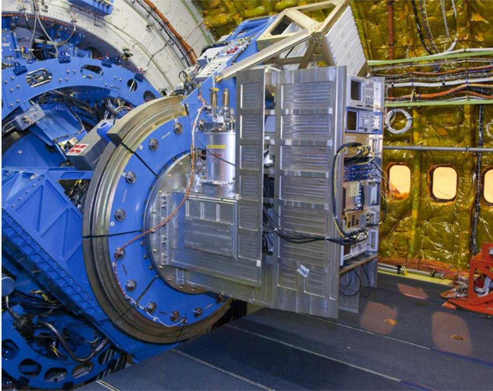
**Figure 5.** The German GREAT instrument mounted at the instrument port of the SOFIA telescope. GREAT can simultaneously operate two receivers, each of them housed in a separate cryostat. One of the cryostats is visible in the figure, the other one is hidden by the instrument support structure. The instrument port is surrounded by counterweight plates (GREAT Team<sup>©</sup>).
