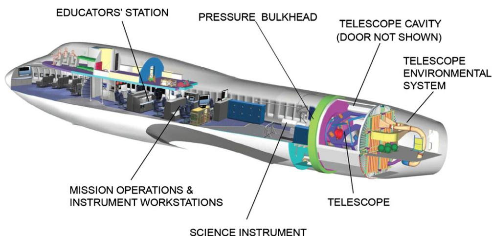
**Figure 3.** A cutaway schematic of the SOFIA observatory. The pressurized cabin is in front of the pressure bulkhead. The telescope looks out of the left side of the airplane. The light for the scientific instrument is fed through the Nasmyth tube, which goes through the bearing. An environmental control system prevents condensation during descent when the door is closed after a night of observations.
