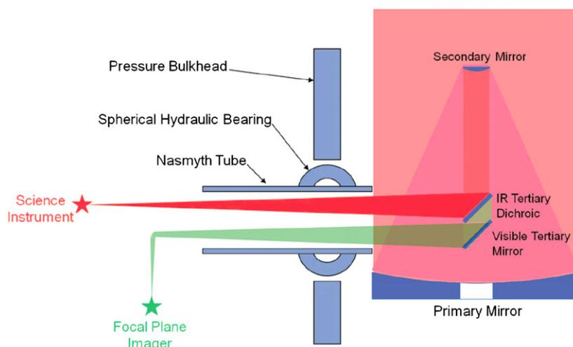
**Figure 4.** A schematic of the optical system of the SOFIA telescope. Everything left of the bulkhead is contained in the forward pressurized crew cabin, while everything to the right is contained in the open telescope cavity.
