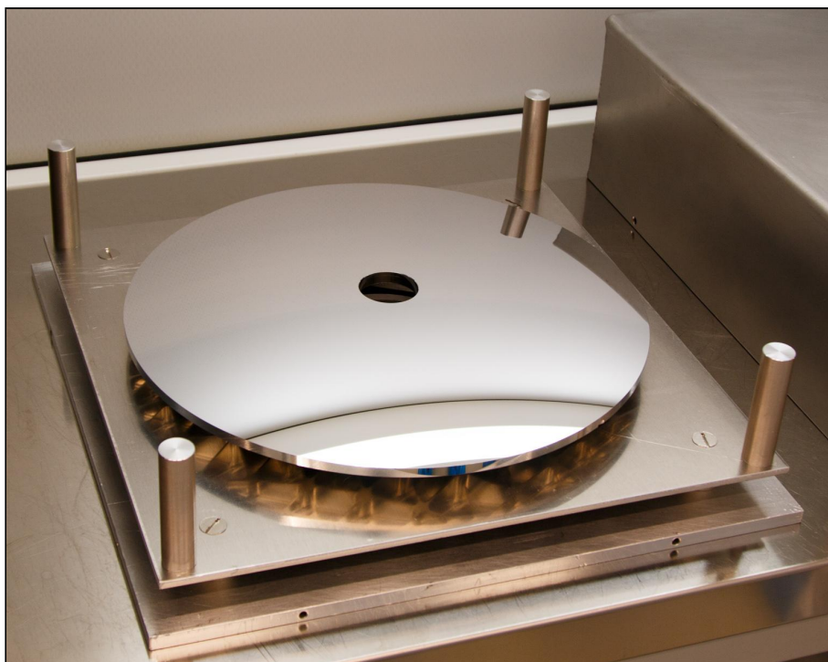
Figure 7. The finished backup aluminum secondary mirror.
